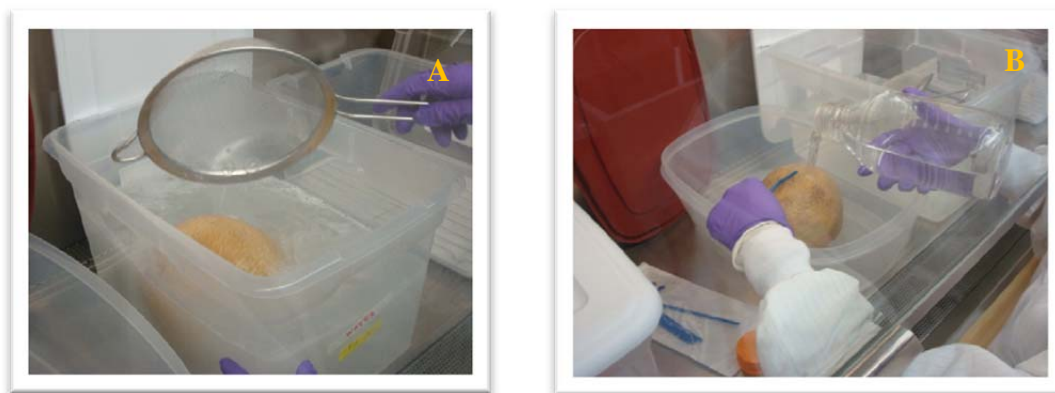
Figure 5. Washing procedures used for cantaloupes treatments. A) use of a disinfected metallic colander to remove cantaloupes from washing solution, B) rinsing step after washing treatment
